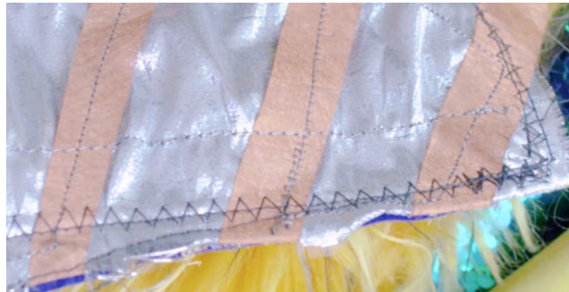
Figure 4 © Safety Third Productions: Copper fabric is made into interactive panels.
