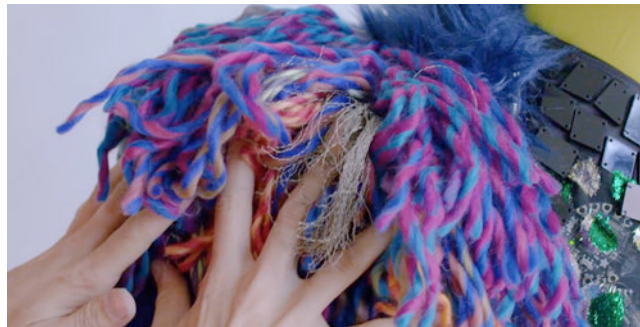
Figure 5 © Safety Third Productions: Conductive thread is tufted into shaggy yarn.
